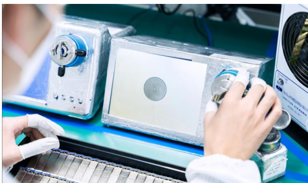
Optical endface inspection
