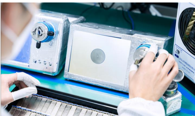
Optical endface inspection
