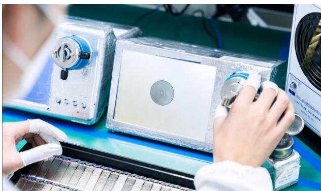
Optical endface inspection
